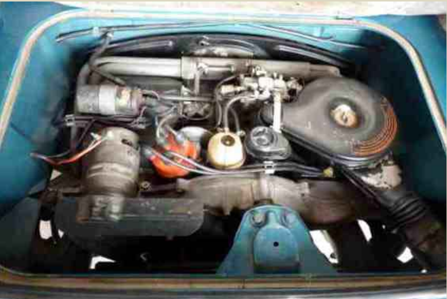
Below: early-1962's had no oil breather tube so the hole in the air cleaner is plugged with an ivory plastic plug.
